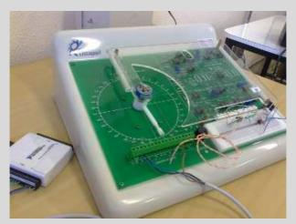
■ Lab Control — research on the theory of control systems: torsional apparatus.
